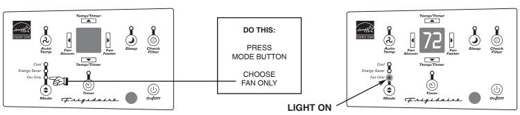
**Note:** Use this function only when cooling is not desired, such as for room air circulation or to exhaust stale air. (Remember to open the vent during this function, but keep it closed during cooling for maximum cooling efficiency.) You can choose any fan speed you prefer. (Except "Auto Temp").
